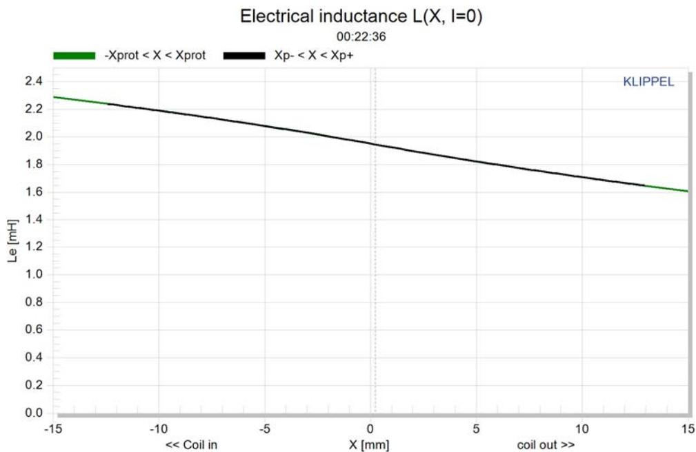
Figure 10:  $L(x)$  measurement of a traditional speaker
