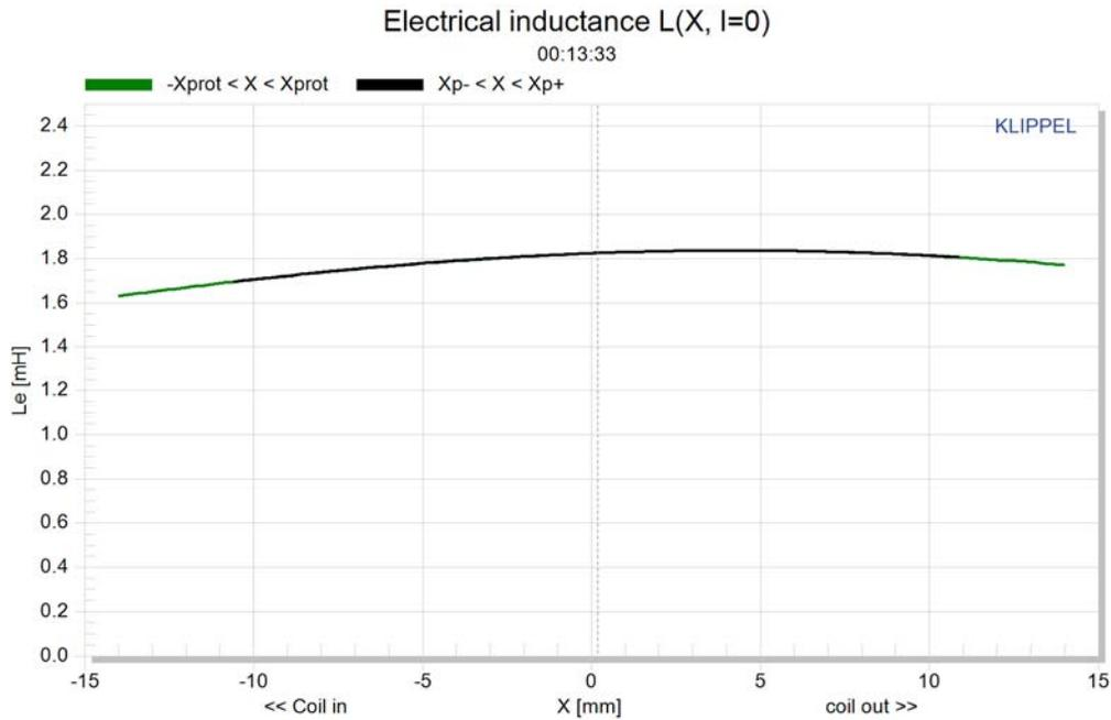
Figure 9:  $L(x)$  measurement of a Tetracoil speaker
