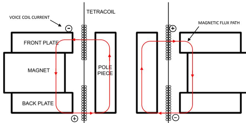
Figure 5: Tetracoil motor showing magnetic flux path flow
