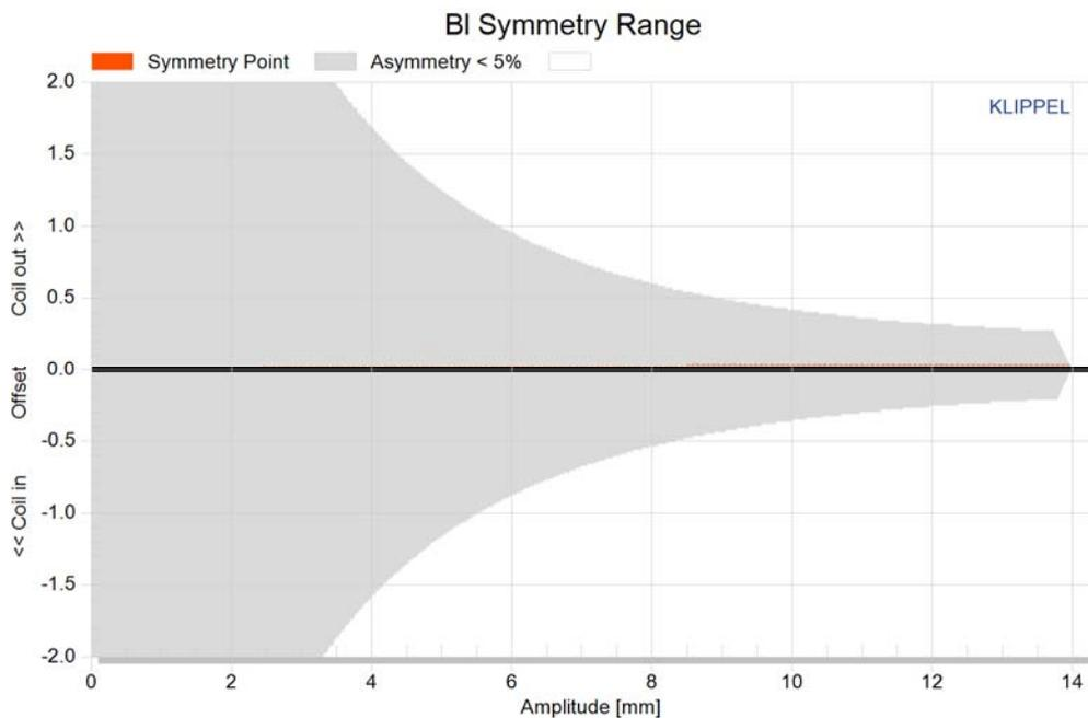
Figure 8:  $Bl$  Symmetry range measurement
