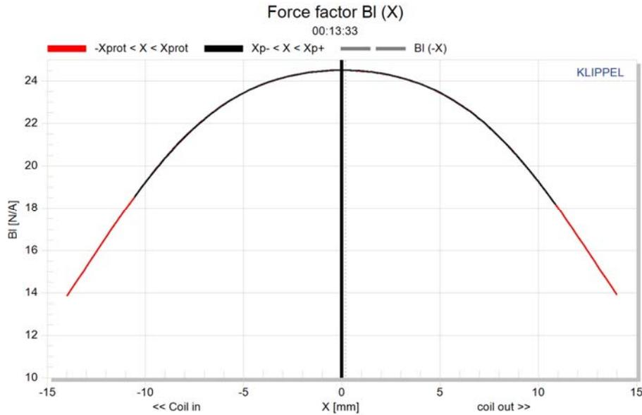
Figure 7: Tetracoil speaker  $Bl(x)$  measurement
