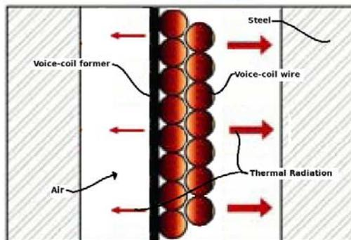
Figure 2: Traditional voice-coil wound outside of the former
