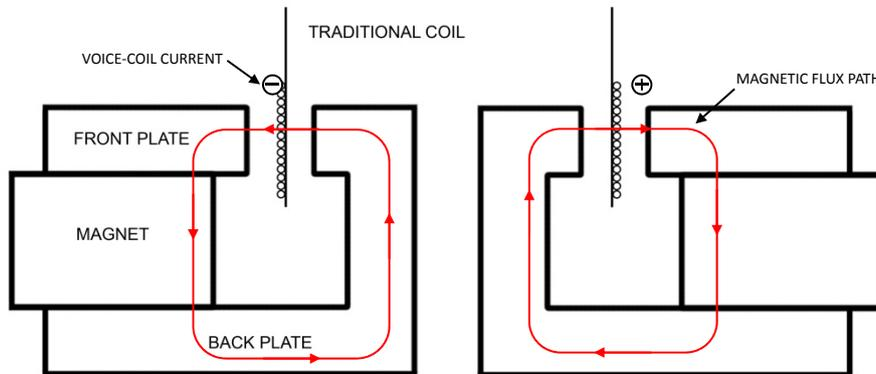
Figure 1 Traditional magnetic circuit with conventional voice coil
