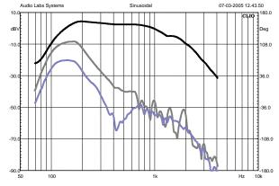
Figure 35: 500-type **with AIC**, driving current response & distortion
