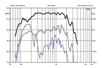
Figure 30: Standard 500-type, response and distortion
