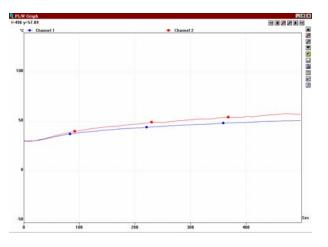
Figure 57: Difference in temperature after about 8 minutes at <sup>1</sup>/<sub>4</sub> of power between the AIC-equipped speaker (the upper curve) and the same speaker but equipped with a copper shorting ring in the gap (lower curve).
