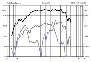
Figure 39: 600-type with AIC, response and distortion
