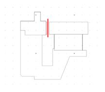
Figure 3: Model of a 500 type magnetic circuit with a shorting ring in the gap instead of the A.I.C. coil
