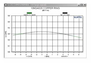
Figure 54: Le vs. displacement in a 500-type speaker with the ring in the gap
