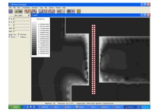
Figure 12: 500-type normal 250Hz - shot 2 - J [A/m^2]
