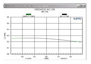
Figure 55: Le vs. displacement in a 500-type speaker with AIC connected
