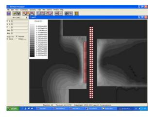
Figure 16: 500-type 250Hz with AIC, shot 3 - J [A/m^2]
