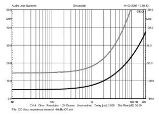
Figure 51: Impedance curves of the blocked speakers: the impedance of the **voice coil** (black) and the impedance of the **AIC coil** (gray curve)
