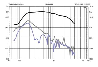
Figure 41: 600-type **with AIC**, driving current response & distortion
