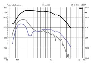
Figure 36: 500-type with **ring under the pole piece**, driving current response & distortion
