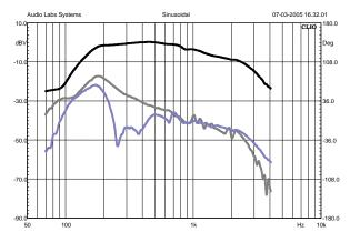
Figure 40: **Standard** 600-type, driving current response & distortion
