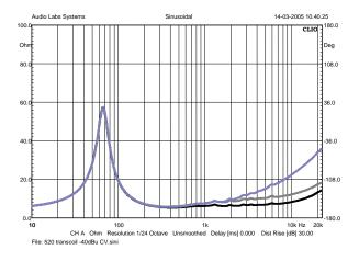
Figure 49: Free air impedance measurement over a 600type loudspeaker: **AIC disconnected** (light gray), **AIC paralleled to the voice coil** (black) or **AIC shorted** (dark gray).
