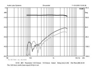
Figure 44: 500-type **with ring under the pole piece**, driving current response & distortion
