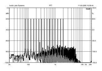
Figure 46: driving current FFT multi-tone test over a 500-type **with AIC** (gray) and without it (black).
