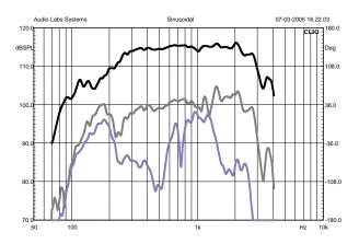
Figure 38: Standard 600-type, response and distortion
