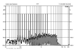
Figure 48: driving current FFT multi-tone test over a 500-type **with a ring under the pole piece** (gray) and without it (black).
