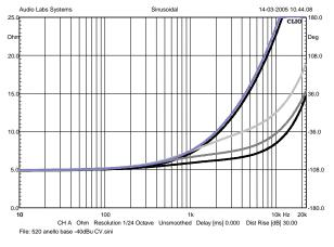
Figure 50: Impedance curves of the blocked speakers
