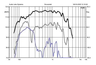
Figure 31: 500-type with AIC, response and distortion
