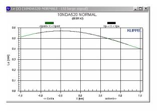
Figure 52: Le vs. displacement in the standard 500-type
