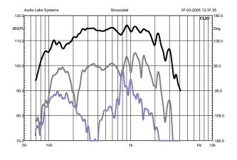
Figure 33: 500-type with ring in the gap
