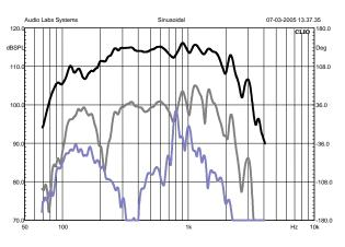
Figure 32: 500-type with ring under the pole piece
